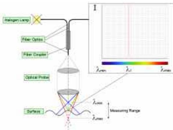
*Principle of chromatically coded confocal measurement*
