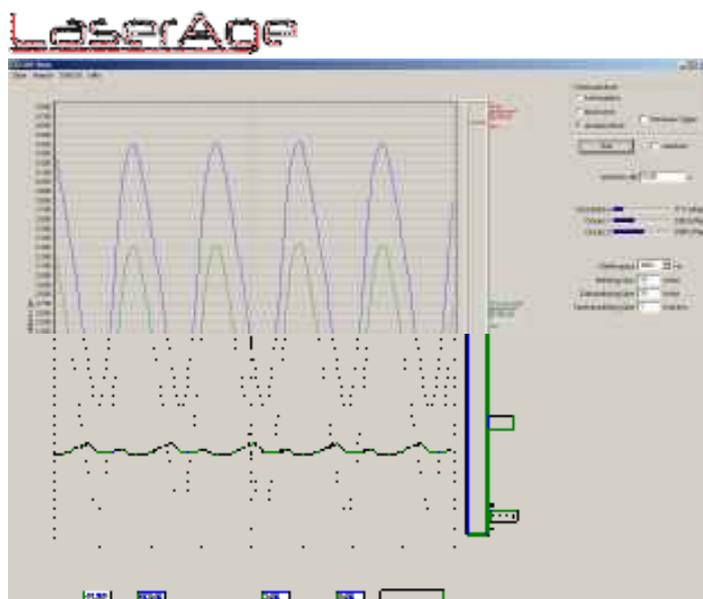
*The comprehensive software package evaluates the measured data conveniently. The example here shows simultaneous evaluation of wall thickness and roundness on a glass bottle*
