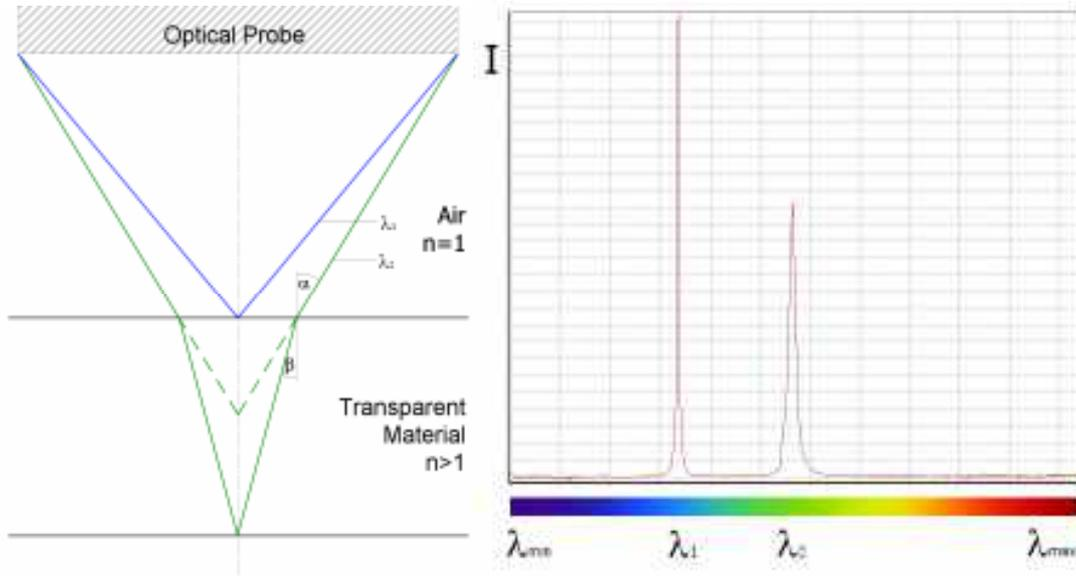
*Beam path and spectrum in a glass thickness measurement. This also enables statements to be made about the object's roundness.*
