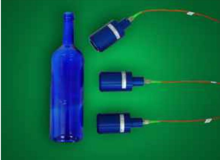
*Coloured glasses are no problem: The arrangement of the measuring heads for a wall thickness measurement is shown here.*
