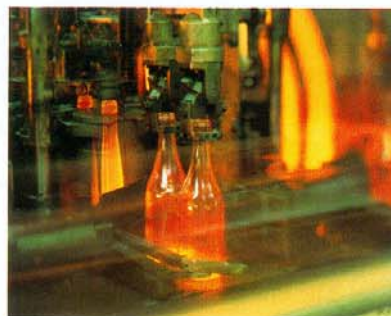
Streaking effects on glowing glass bottles have no influence on the measurement.
