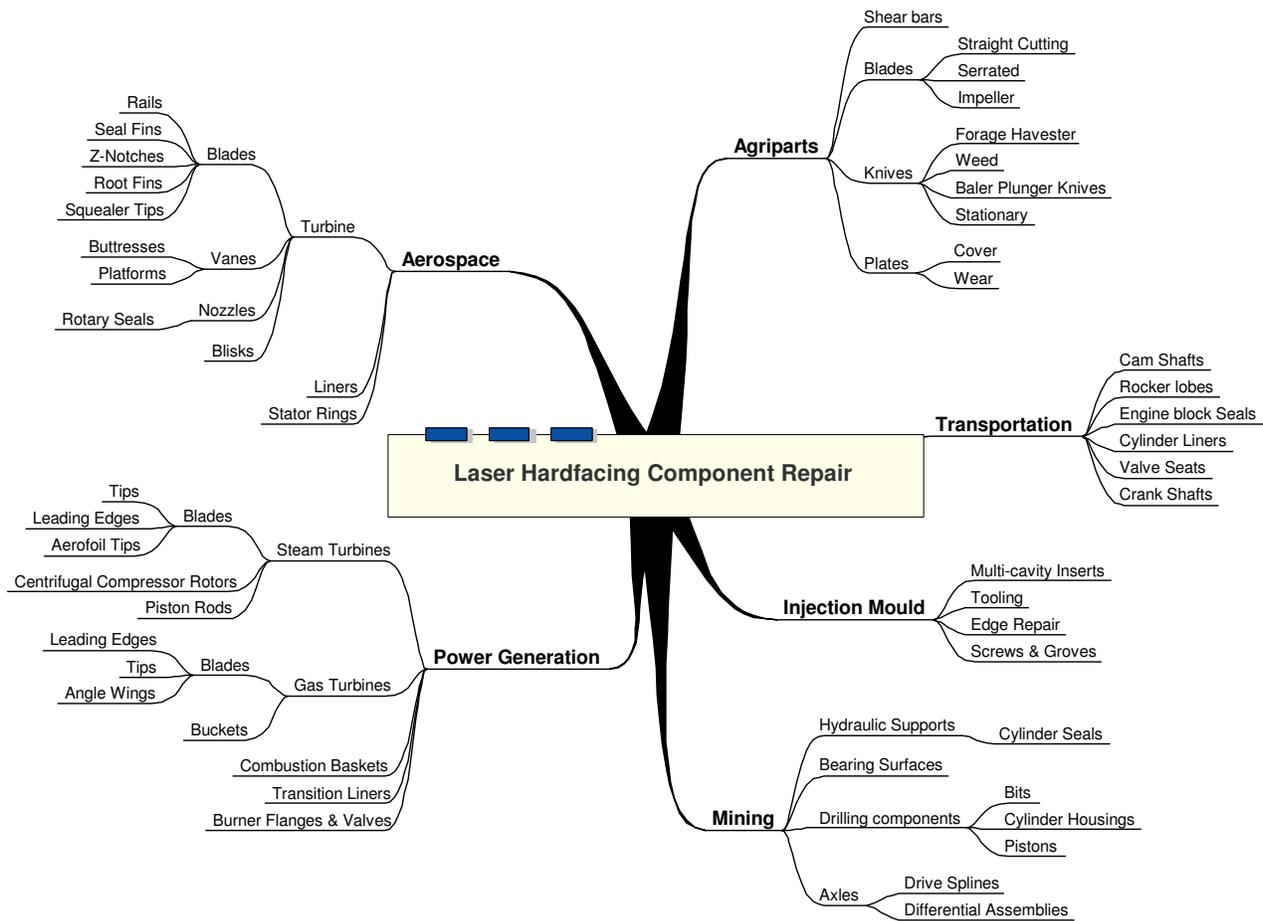
Figure 2; an extensive list of component wear parts that are suitable to the laser cladding (hardfacing) process.
