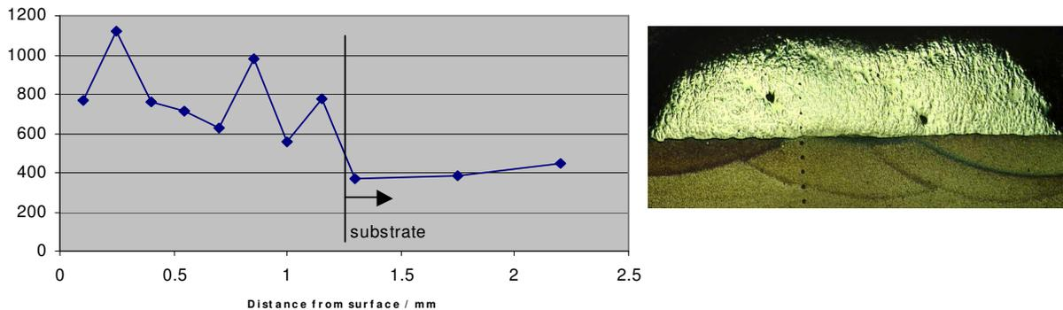
Figure 5; Graph of Hardness of WC + Ni base binder material laser hardfaced onto a cast Fe substrate.
