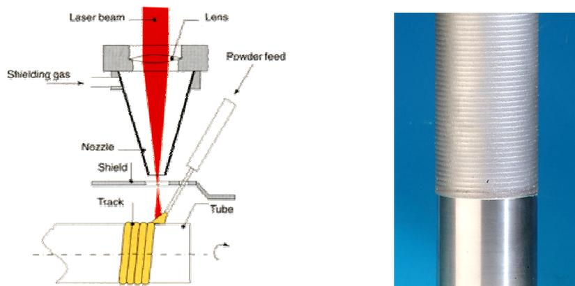
Fig. 1(a) Schematic of the Interaction Zone (b) Shaft Cladding
