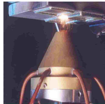
Overhead Cladding (designed by ILT)
